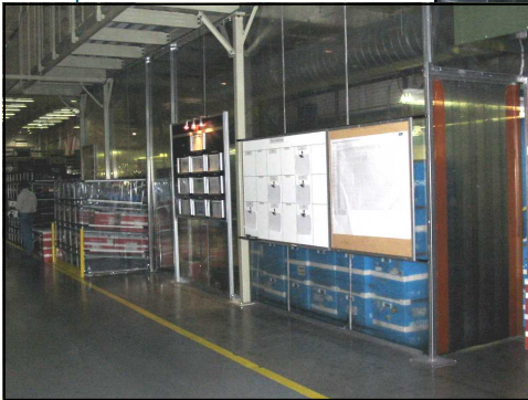
Parts load/unload work station enclosing an area under a mezzanine structure.
