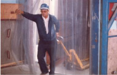
Overlapping strips control temperature, welding flash, dust & fumes, and noise while allowing for easy access for people and equipment.
