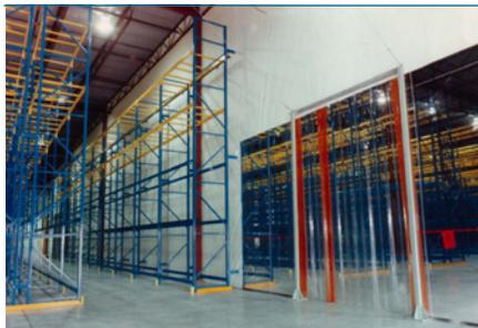
Floor to ceiling partitions to divide an entire facility, enclose temperature-sensitive environments, separate shipping/receiving from manufacturing, section off different product categories or work process, or temporarily subdivide and sublet a facility.
